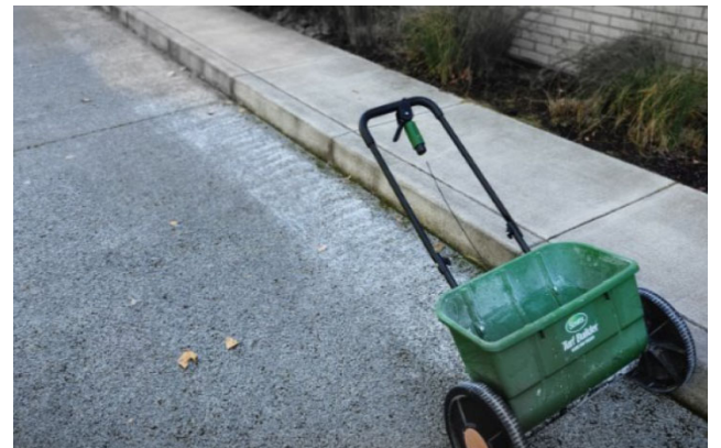
Applying a thin coating of baking soda with a spreader (1900 square feet per 50-pound bag) killed the moss within hours.
