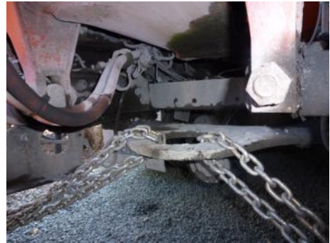
Center mounted tow ring works best.
